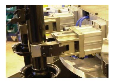
closing torque range from 24 to 350 Nm with a massive closed retention force of 773 Nm for the largest of the four sizes, well capable of handling heavy drive shafts or similar.
